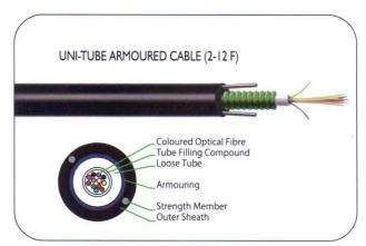
Colour coated optical fibers are put in a loose tube filled with Thixotropic jelly. Two high tensile Steel Wires (or FRP Rods) are embedded in the polyethylene sheath for getting desired strength and rigidity in the cable. Additional peripheral strength members may be included to provide additional pulling tensile strength.
